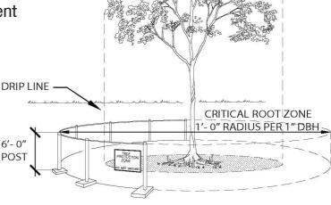
TREE PROTECTION ZONE IS AT THE EDGE OF THE CRITICAL ROOT ZONE OR DRIP LINE, WHICHEVER IS GREATER
